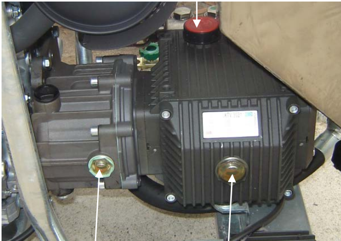
Gearbox sight glass
